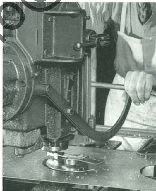
3 Circular aperture cutting, using adjustable rotating guide.
