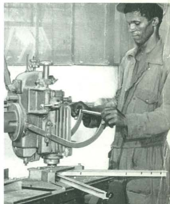
4 Removing flash from non-ferrous window frames
